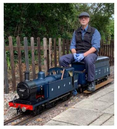
Tank Engine, to run on standard 7 ¼" gauge track. I drew up the designs on computer, based on measurements and photographs taken from the full-size engine 47406 which is based on the Great Central Railway at Loughborough. The models are about four feet long (1,200 mm) and 13 inches wide (330 mm), weighing about 400 lbs (180 Kg) in working order. They are capable of hauling up to about a ton on level track, so roughly ten adults, riding on our CADMES coaches.
